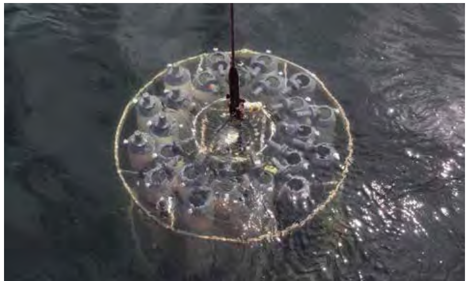
A CTD (conductivity, temperature, and depth) rosette taking water samples in Baynes Sound, British Columbia. Photo: Dan McPhee (DFO)
