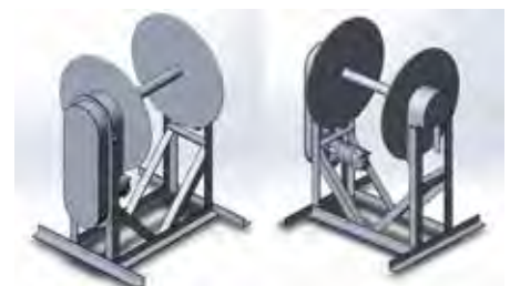
Design drawings of a rotating drum with a hydraulic motor. Photo: Daniel Leblanc (Merinov)
