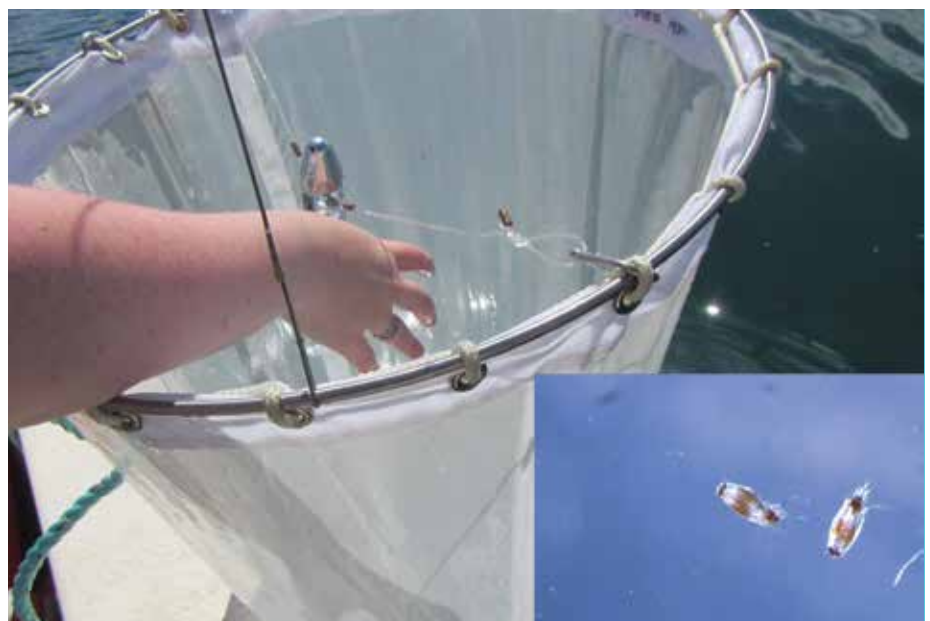
Plankton net with flow meter used to sample sea lice larvae (inset) in and around salmon farms in the Bay of Fundy. Photo: Shawn Robinson (DFO)
