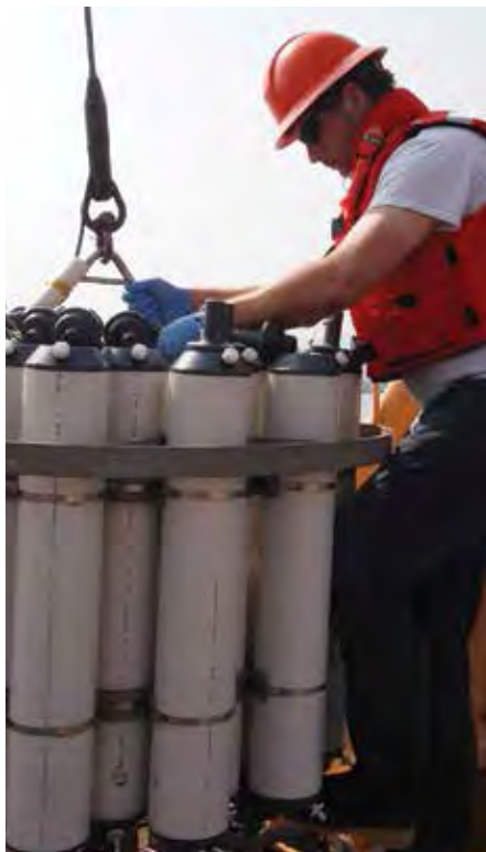
Dan McPhee setting the firing mechanism on a CTD rosette to collect samples in Baynes Sound, British Columbia. Photo: Terri Sutherland (DFO)
