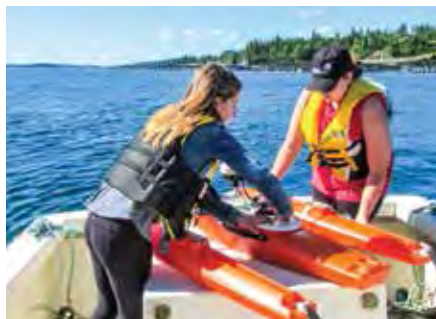
Taryn Minch (UNBSJ) and Adena Peters (UNBSJ) monitoring an acoustic Doppler current profiler (ADCP) while it measures the current speed and direction of the water in the water column around an aquaculture farm in the Bay of Fundy. Photo: Shawn Robinson (DFO)
