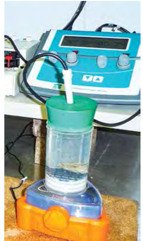
Respirometry system for measuring the physiological status of bivalves. Photo: Lisandre Gilmore-Solomon (Merinov; CÉGEP de la Gaspésie et des Îles)
