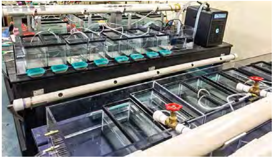
Exposure tanks for Spot Prawn ( Pandalus platyceros ) for toxicity experiments under multiple stressor conditions. Photo: Feng Lin (SFU)
