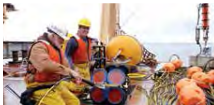
Final checks prior to the deployment of a current meter mooring from the CCGS John P. Tully off the west coast of Vancouver Island are made by Lucius Perreault and Roger Savoie. Data collected by a network of moorings are used to validate the currents simulated by the FVCOM hydrodynamic model. Photo: David Spear (DFO)
