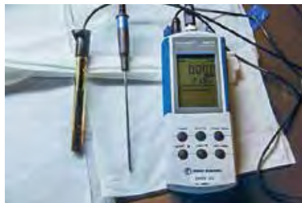
Sulfide probe, temperature probe, meter (left to right). Photo: Fred Page (DFO)
