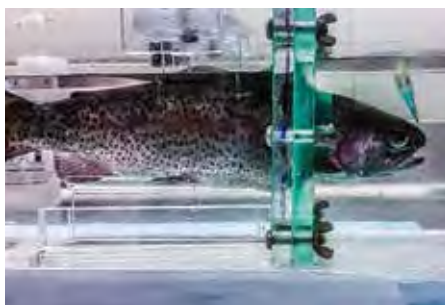
Phosphorus-deficient Rainbow Trout in holding to measure specific absorption through the gills. Photo: Émilie Proulx (U Laval)
