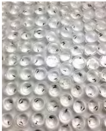
Pill cups loaded with individual stage V lobsters before exposure to spiked sediment with ivermectin and emamectin benzoate (via commercial formulations). Photo: HMSC
