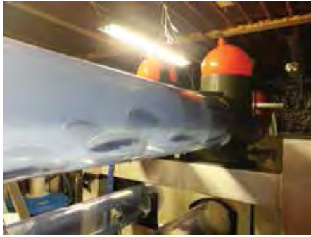
Exercise training Atlantic Salmon ( Salmo salar ) in the Brett-type two-channel swimming tunnel. Photo: Yangfan Zhang (UBC)
