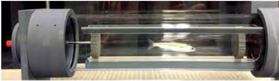
Swim tunnel used for assessing fish swimming performance (critical swimming speed [Ucrit]) following exposure to chemotherapeutants. Photo: Feng Lin (SFU)
