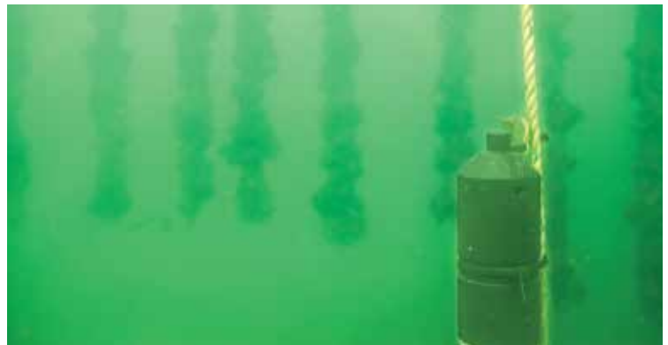
Mussel socks with a hydro-acoustic receiver used to detect ultrasonic signals emitted by acoustic transmitters affixed to lobsters and crabs in Malpeque Bay. Photo: Chris McKindsey (DFO)
