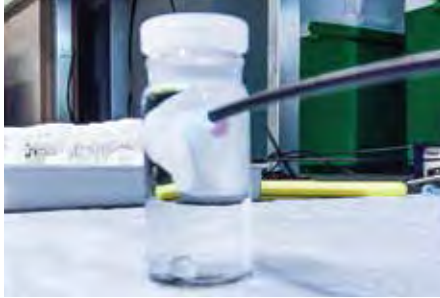
Miniature respiration chamber holding a filter (0.2 µm pore size) coated with bacteria and seston from a sample. The pink dot is an oxygen optode that reads oxygen levels over time inside the vial when pulsed with blue light from outside the vial with the black fibre optic probe. Photo: Shawn Robinson (DFO)
