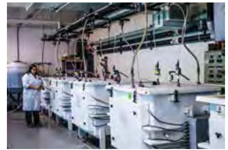
NRC Technical Officer, Jenny MacPherson, poses with NRC-developed "Brite-Box" photobioreactors (>10,000 L production capacity). Photo: Scott MacQuarrie (NRC)
